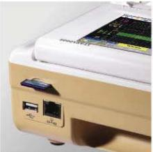
Support data storage and software upgrading by external USB disk
